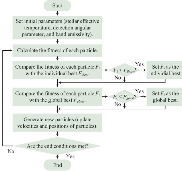
FIG. 2. The flow diagram of our SPSO algorithm.
